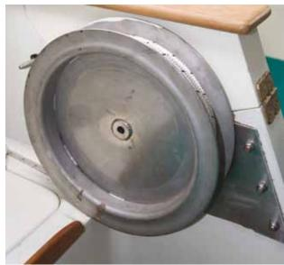
**Facing page:** The outboard is immediately accessible in the generous full-width cockpit. **Above:** Kite looks clean and bright down below; Colin suspects some owners may want a little more brightwork. The 10:1 centreplate winch is easily accessible just inside the main hatch.
