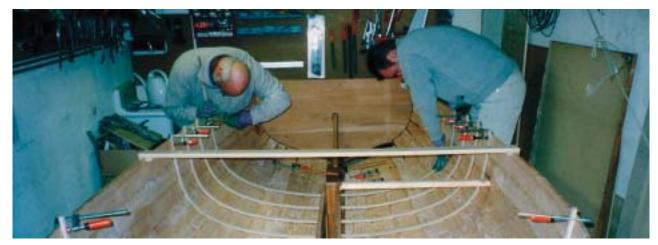
Above: The timbers – frames – were made from green oak which steams very well. My son and I worked as a team, pushing the longest frames into place first so that any breakages might still be able to be used in the bows or beside the c/b case. We made sure of a snug fit at the turn of the bilge. After cooling overnight, the frames were numbered and then removed to allow them – and the inside of the hull – to be sanded down and then given three coats of the French le Tonkinois varnish.
