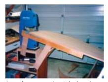
In order to saw the right bevels on edges of the transom, I made up this jig for the bandsaw to hold the mahogany at the correct angle.
