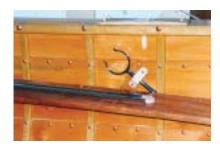
The jib sheets have their own narrow side benches, the rowlock pads and sockets have been fitted, as has a neat stowage arrangement for the rowlocks. The pads are bevelled a little to ensure the rowlock sockets are central so that the rowlock stems clear the planking. Lower supporting blocks for the rowlocks were also fitted.
