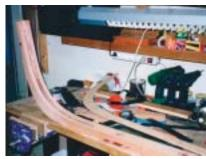
The apron, laminated from 3 layers of mahogany in 3 sections with an inner full-length veneer to hide the joints, was glued with resorcinol.
