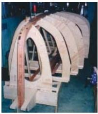
Above: The apron, keel and tapered hog were laminated in situ and fastened to the transom. For this first phase of the build I used resorcinol glue but for the rest I used epoxy for better gap filling. Below: Sheathed with polythene sheet, the apron became the former on which I laminated the outer stem using 10 layers of 5mm mahogany
