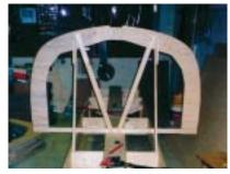
The building jig was fastened to the floor and the structure stiffened by the flat central plank. There were 8 mould frames of 20mm chipboard.
