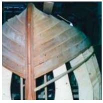
How did I do it? After roving up, I temporarily fixed a round batten on the marks for the next plank which acted as a guide for the plane when planing the bevel. A supporting bar, fixed to the plane to get the correct angle, slid along the round batten.
