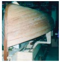
Building Swallow upside down left most space in the workshop. After finishing the planking, I removed most of the building frames and installed the centreboard case. The inside width of the case is 50mm and internal 'rubbing strakes' hold the board central while leaving plenty of space at each side of it so that gravel falls out easily.
