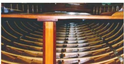
Above: When the varnish was dry, the timbers were re-fitted:rivetted through the lands and screwed down to the hog, taking great care that they were all at 90° to the hog. Note the wedges which support the timbers either side of the hog.
