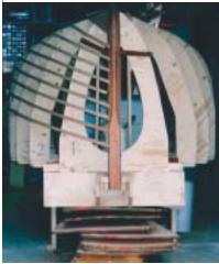
The planking layout is critical to the appearance of a clinker boat: every strake must taper evenly in a natural progression from the mid-section to the ends. Though maths does help, the only way to get it really right is doing it 'by eye' with lining battens. A photograph like this is also useful: you can turn it through 180° to see what she will look like right way up. After studying this particular picture, I re-aligned the fifth batten a little.
