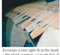
To ensure a nice tight fit at the lands – the plank overlaps – I made lots of peg clamps. I waterproofed the seams between the garboards and the keel and at the hood ends with Sikaflex, the rest were dry-fitted and on launching, there wasn't one leak!
